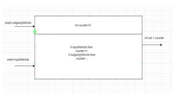
Since there are four sensors installed, one for each direction, we have utilized four vehicle counter components. These components determine the net vehicle count at the intersection and then forward that information to the direction SRC for further processing.
