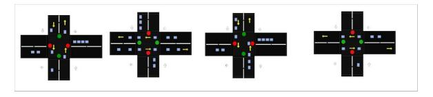
The system is said to be operating in a normal mode when there are no emergency vehicles in the intersection. During this mode, based on the number of vehicles in both directions
