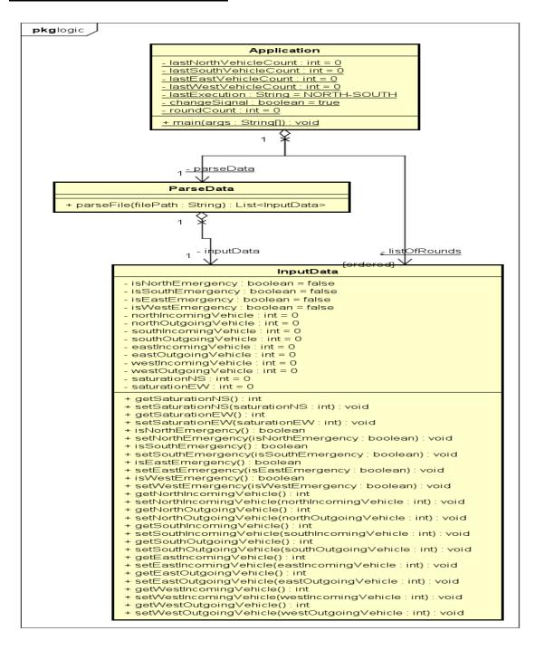
The given class diagram is a subset that focuses on the feature of retrieving vehicle data from sensors. To achieve this, the data is obtained from a text file. The process involves invoking the "read" function from the Application class, retrieving the file from the resource folder, and parsing it into a format that can be easily read by the Application class.
