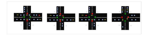
When an emergency vehicle approaches an intersection and when its direction is having a green light, the controller does not change the light for 20 seconds. Here it is also assumed that other civilian vehicles would facilitate the emergency vehicle by giving its right of way.
